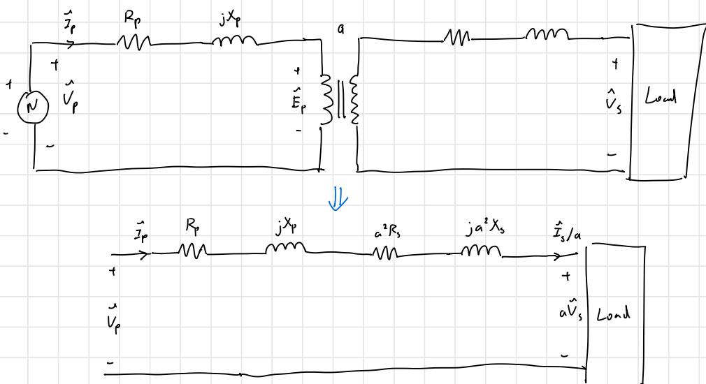
$$\text{a. } a = \frac{N_p}{N_s} = \frac{2400}{240} = 10, \quad 20 \text{ kVA} = \text{maximum load}$$
